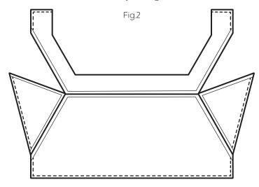
The assembled roof should sit solidly on the main structure. Reinforcement with small scrap wood blocks glued to the inside or the use of hot glue at the inside joints in addition to white glue will add extra strength.
